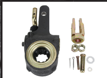
SLACK ADJUSTER, AUTOMATIC, 5.5", GUNITE STYLE
